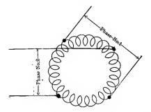
FIG. 65. Diagram of interconnected or closed-coil two-phase winding. Any closed winding may be thus connected.
